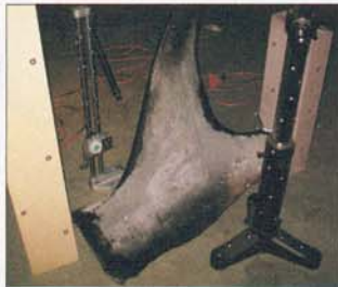
Preparing a frozen dorsal fin for laser scanning, using target points to align multiple scans.
