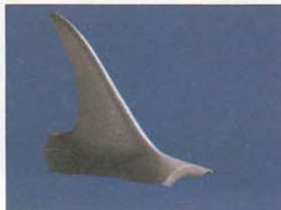
STL output created from point cloud data captured with a non-contact digitizer.
